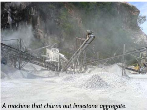
A machine that churns out limestone aggregate.
